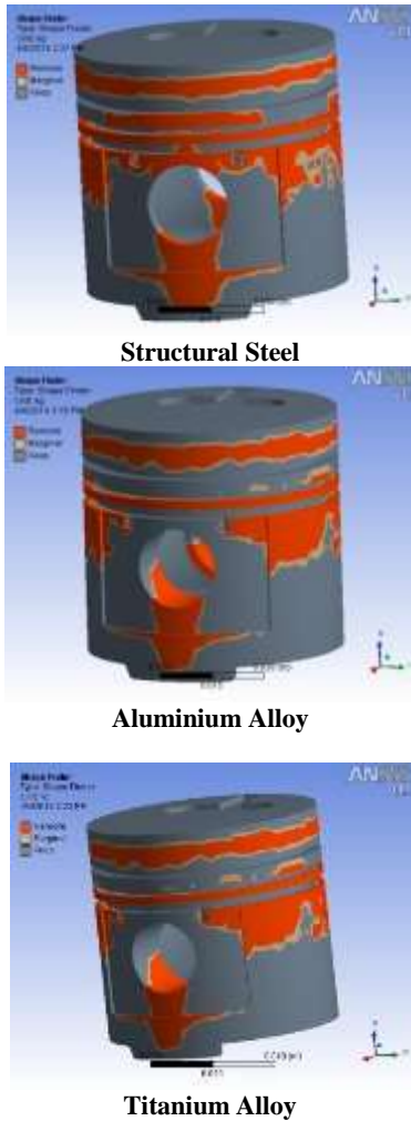
Fig 5.5 Comparison between Shape optimization Table 5.1&5.2 shows final results for structural Steel, Aluminum Alloy and Titanium Alloy in Tabular form.
